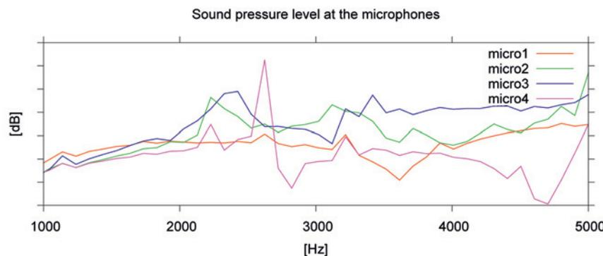
Fig. 4: Frequency response functions at remote microphone positions
