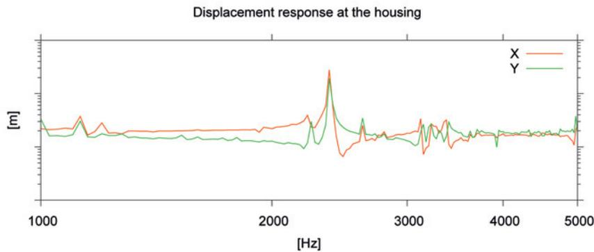
Fig. 3: Results of displacement spectrum of the housing
