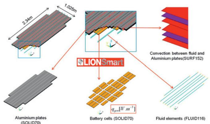
Fig. 1: The overview of electrothermal simulation of a battery pack
