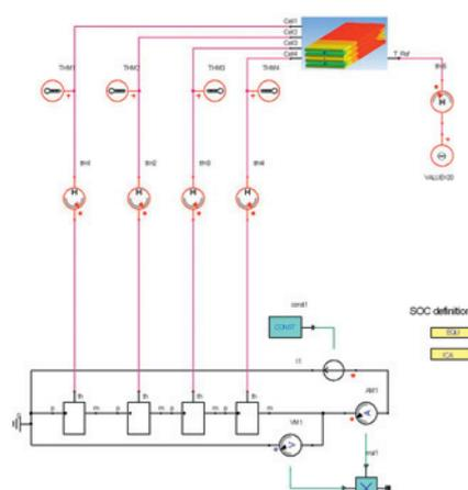
Fig. 4: Electrothermal simulation of the battery pack at system level.
