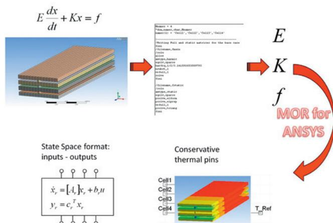
Fig. 3: Model reduction process.
