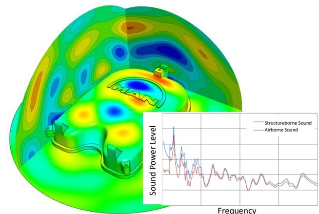
Sound pressure contours and frequency response function of sound power level for a selected engine component
