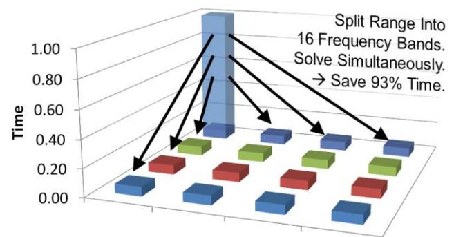
Significant reduction of elapsed time for acoustic simulation by means of HPC parametric distribution of harmonic analysis
