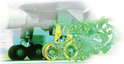
Vortical structures generated by an aircraft landing gear visualized using deformation isosurfaces colored by velocity magnitude
