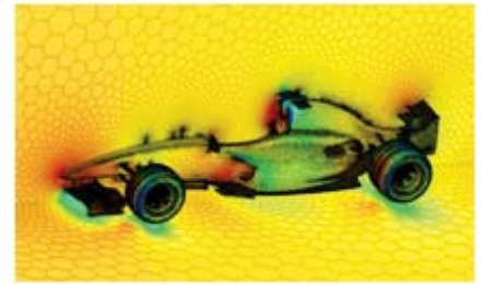
Polyhedral mesh and pressure distribution on an F1 car post-processed using ANSYS CFD-Post software
