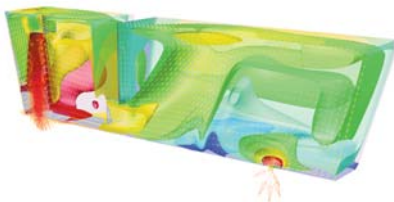
Turbulent kinetic energy in a steel tundish during a continuous casting process
