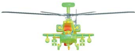
Contours of pressure on a helicopter in hovering flight mode
