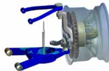
Transient analysis of rigid/flexible suspension mechanism using kinematic joints, springs and contacts
