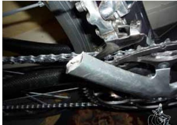
Bicycle crank shaft broken due to fatigue
