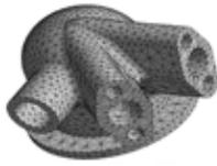
*Automatically generated mesh for finite element analysis*
