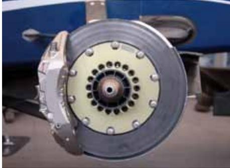
Carbon fiber disc brake
